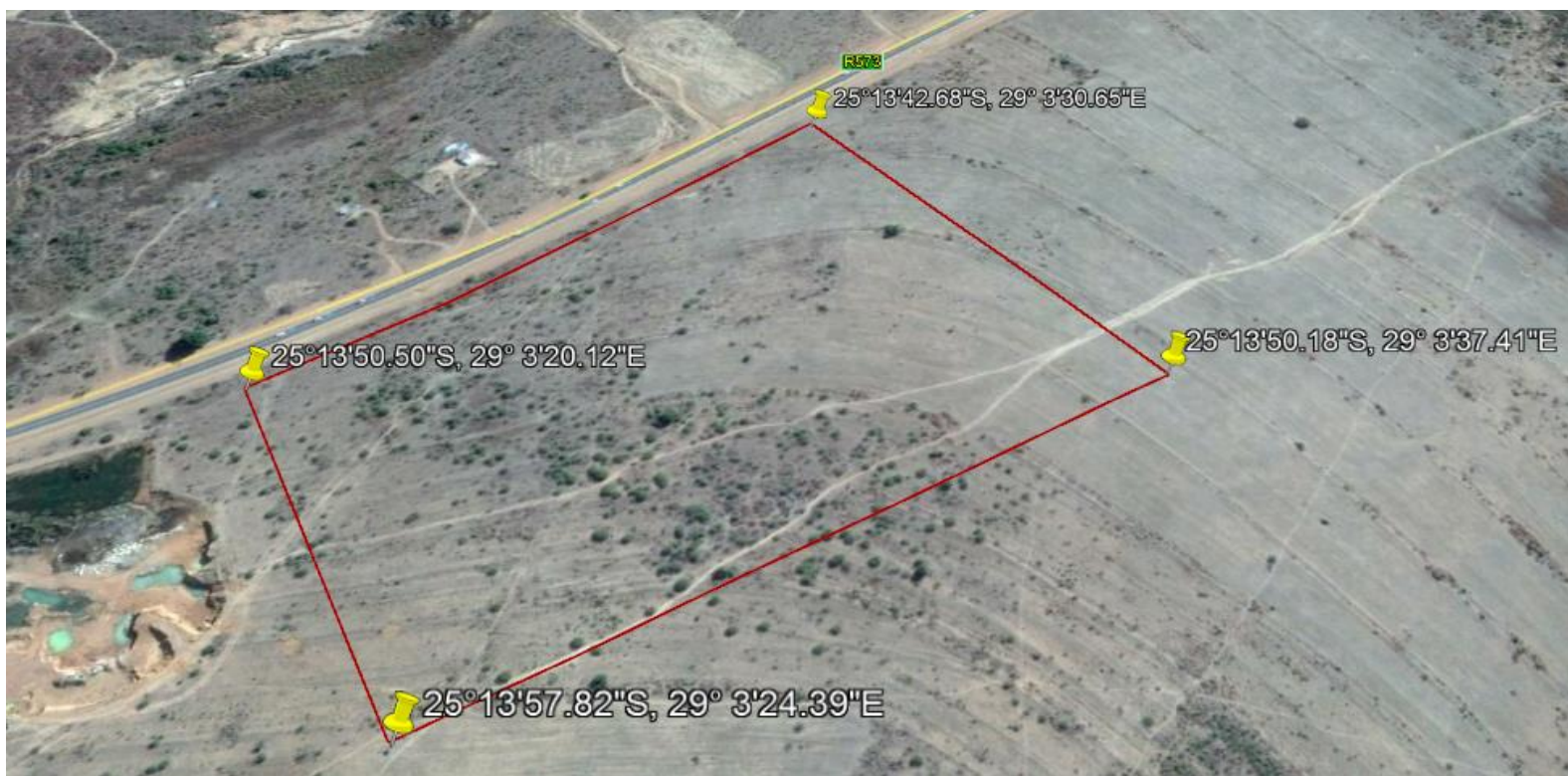
Figure 6: Coordinates of the corner points of Borrow Pit 3
