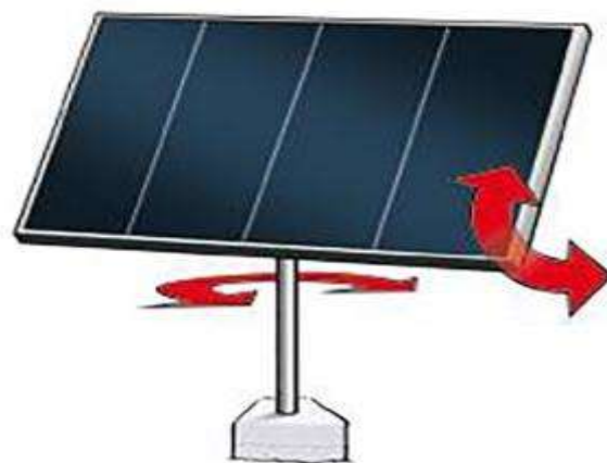
Figure 4.2.: Diagrammatic representation of a typical horizontal/single-axis tracking system and its degrees of rotation.
