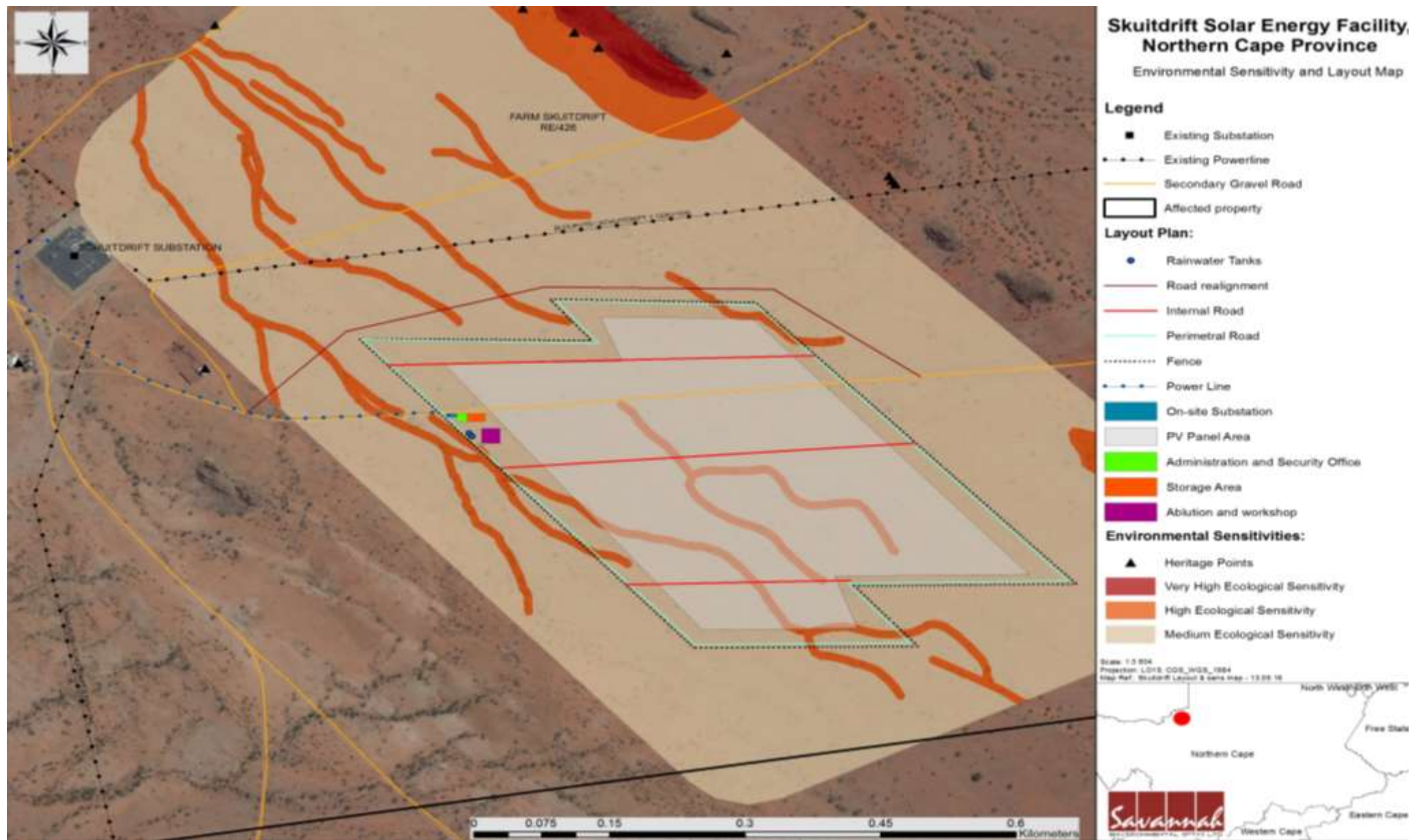
Figure 8: Map depicting the Ecological Sensitivity of the site overlain on the proposed preferred layout
