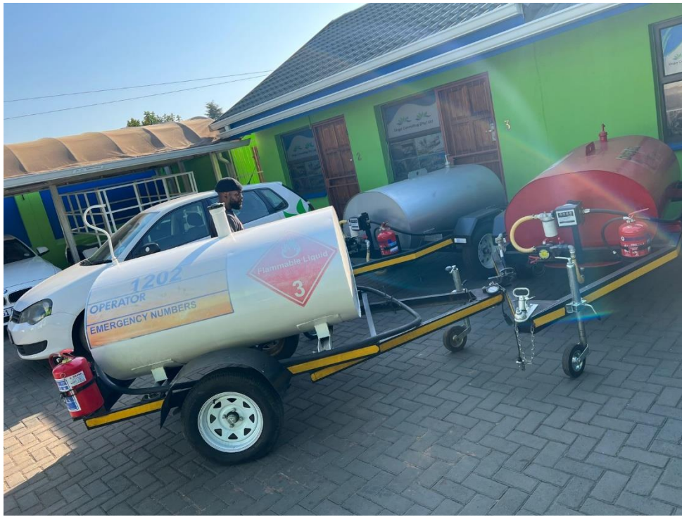
Figure 9: Diesel storage tank.
