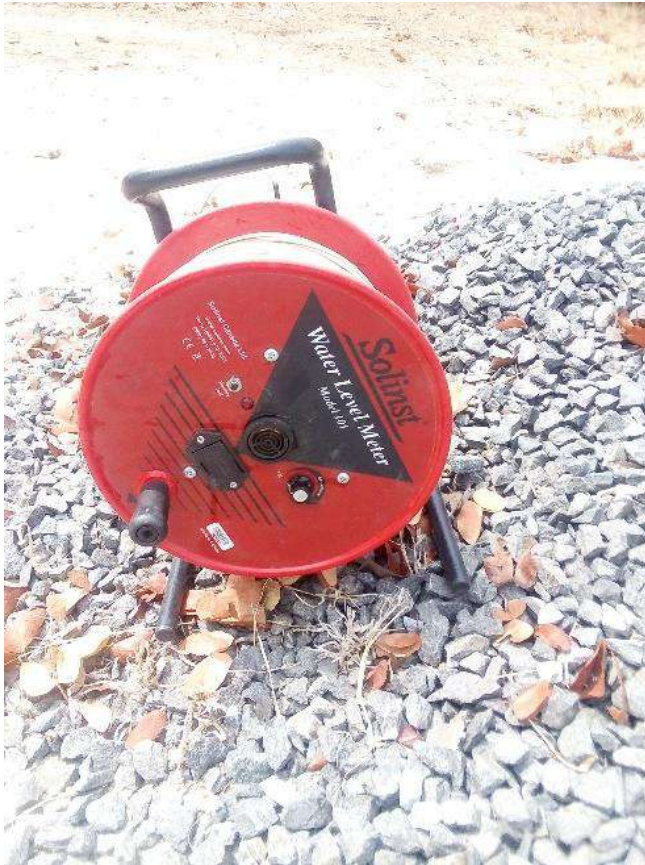
Figure 13: Water level Meter
