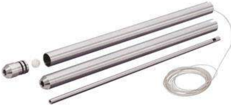
Figure 2: Stainless steel bailer, picture extracted from ( Solist, n.d. ). A bailer uses a simple ball check valve to seal a sample of the groundwater table at the bottom to raise it up
