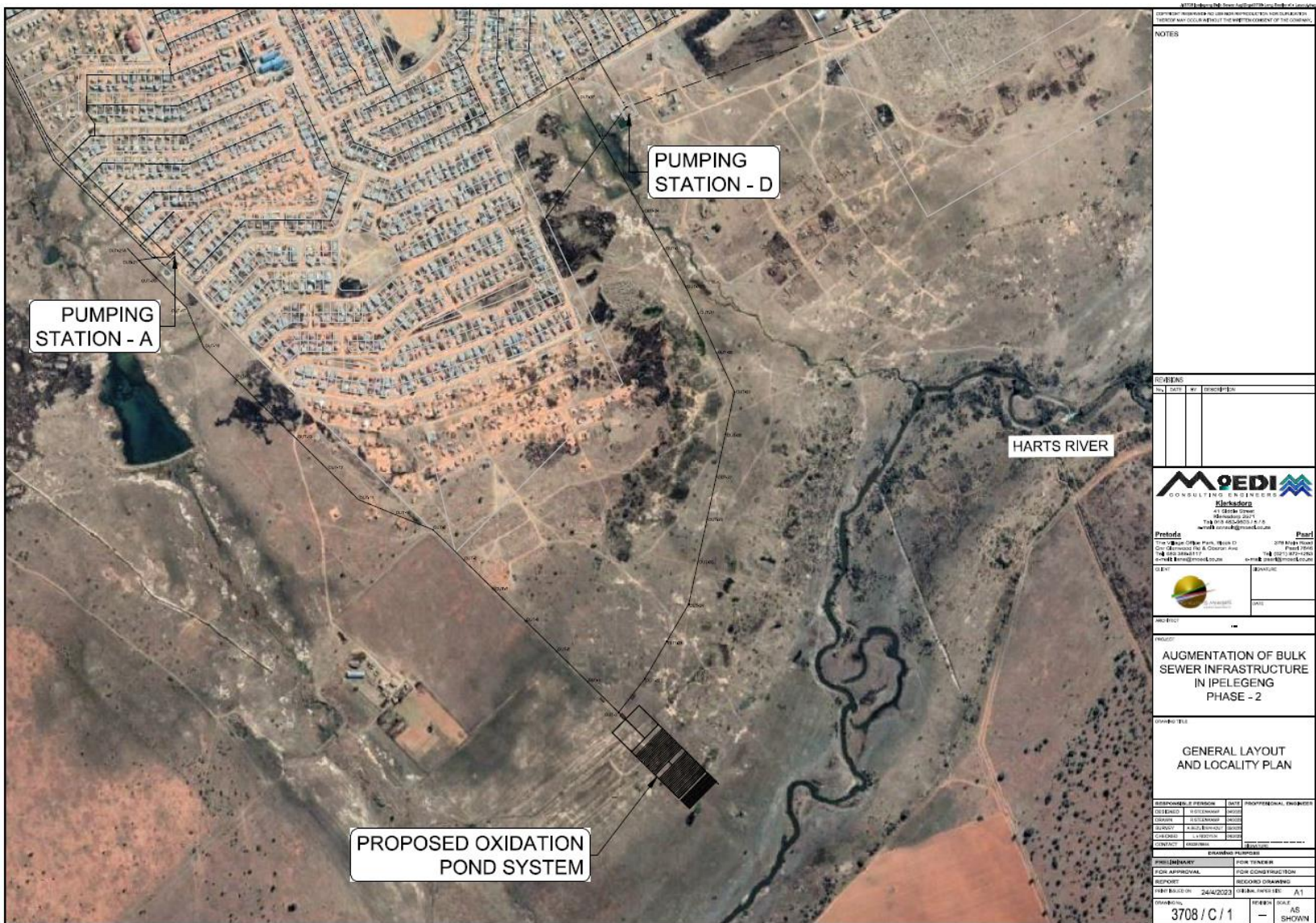
Figure 3: Layout Map of the proposed Sewer lines and Oxidation Pond System, Ipelegeng, North West Province
