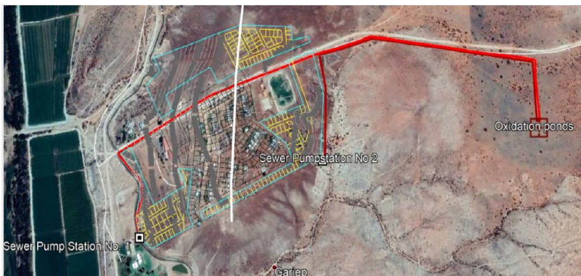
Figure 6. Proposed bulk sewerage system if required.
