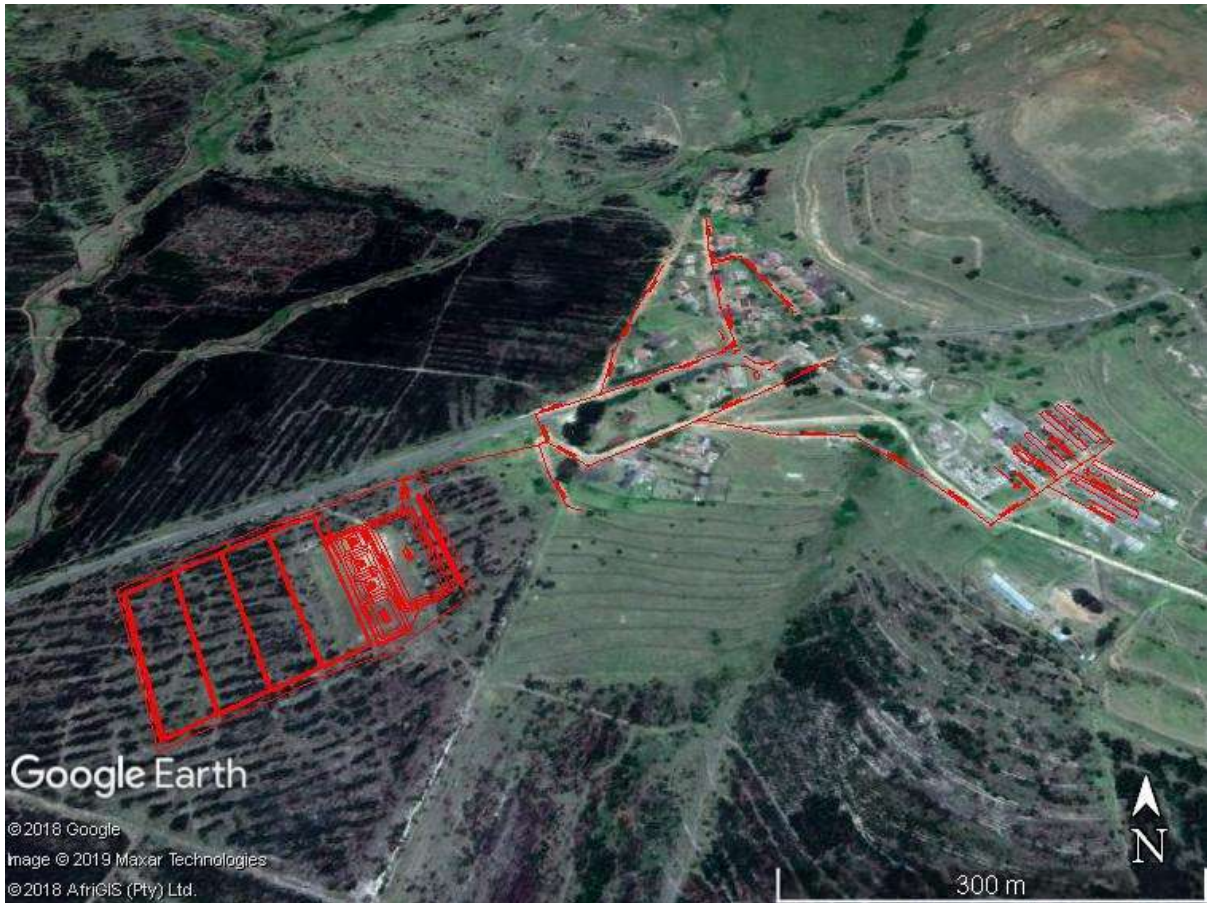
Figure 1: Google Earth map of the proposed upgrading of the sanitation system in Bhokwe Village, Bhokwe Community, Ward 05, AbaQulusi Municipality. The red lines indicate the sewer reticulation and the sewer oxidation ponds.
