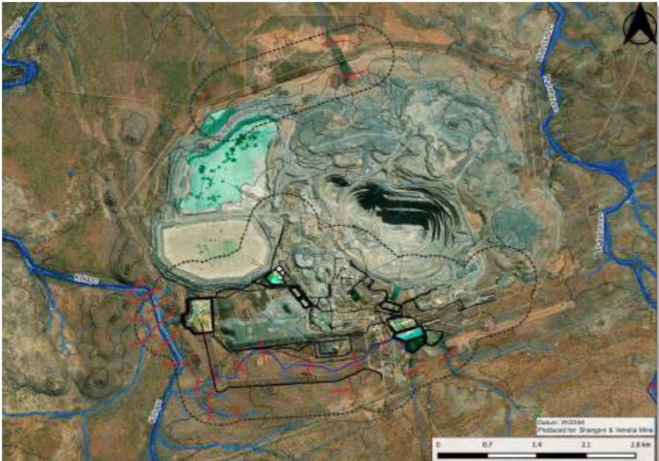
Figure 9: Drainage lines and areas of surface water in the surrounds of the study sites
