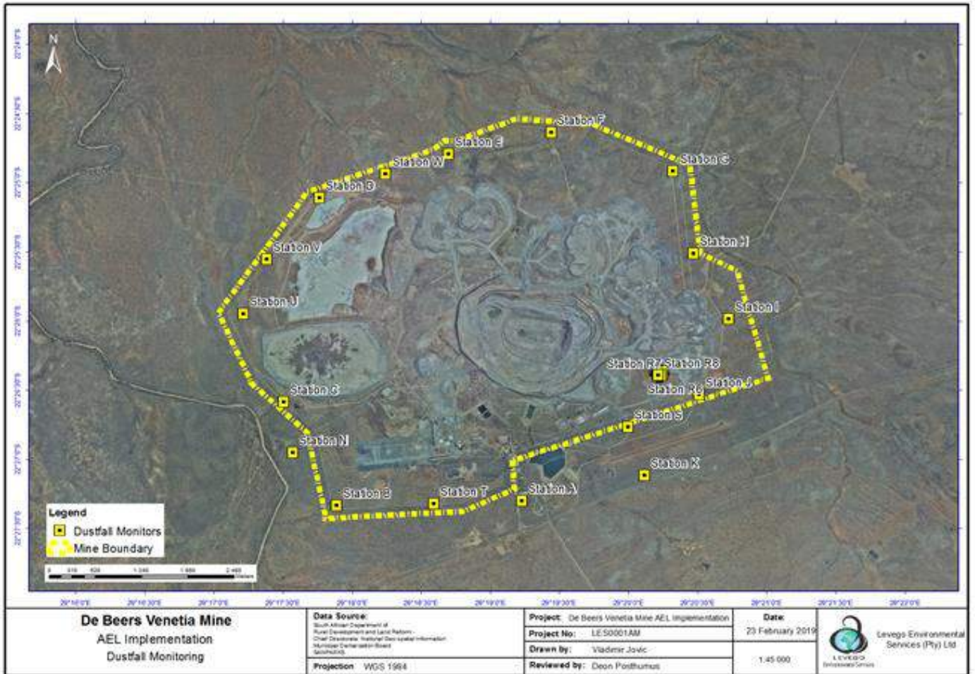
Figure 2: Location of 17 dust fallout monitoring sites along the site boundary of Venetia Mine presented on the satellite image map.
