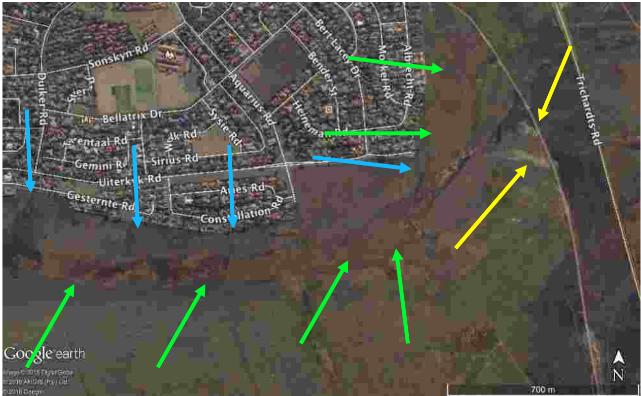
Figure 25 Permanent wetland vegetation (green arrows) in the watercourse on the western side of the site, distinct gold mine tailings spills from pipes (yellow arrows) and storm water signatures (blue arrows)
