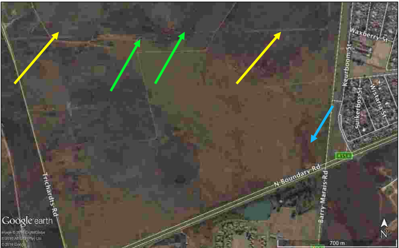
Figure 26 Wetland vegetation, in the eastern side of the site (north: top; south: bottom), associated with storm water signatures (blue arrows) and sewage effluent (green arrows) as well as a distinct pipeline effect (yellow arrows)
