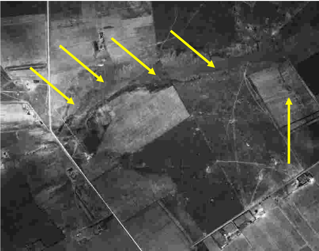
Figure 20 Aerial photograph of the site (1938) with drainage features indicated by yellow arrows
