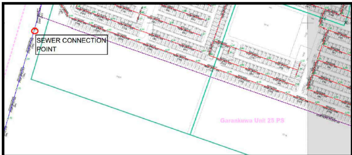
Figure 11: Existing Sewer Layout
