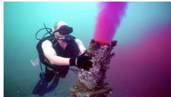
Figure 2-10 Brine nozzle discharge from Australian SWRO plant with the addition of a red dye (rhodamine) to indicate dispersion for the monitoring process
