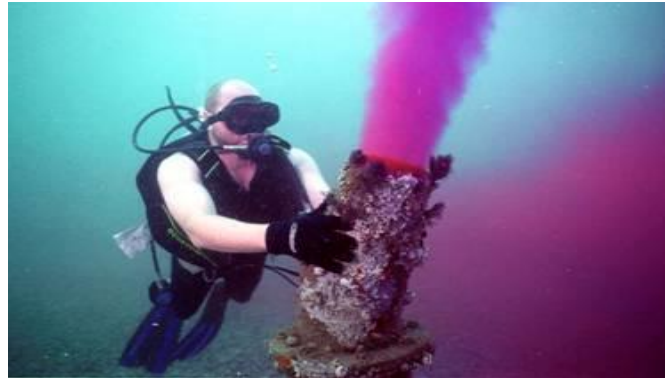
Figure 2-12: Brine nozzle discharge from Australian SWRO plant with the addition of a red dye (rhodamine) to indicate dispersion for the monitoring process
