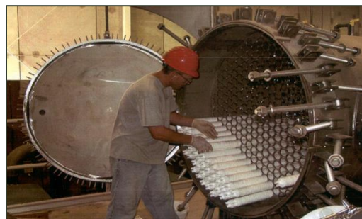
Figure 2-7: A typical cartridge filter arrangement
