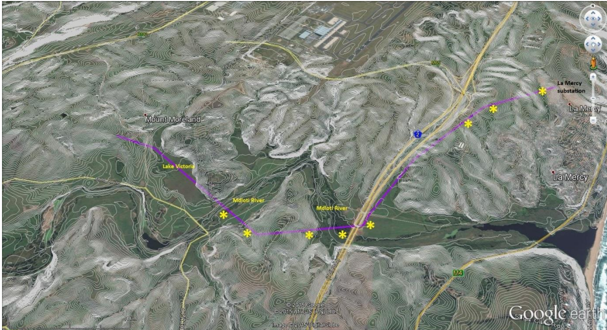
Figure 8-11: Proposed 132 kV Transmission Line alignment (purple line) from La Mercy to substation near Mount Moreland 2m contour lines shown; drainage lines of concern asterisked.
