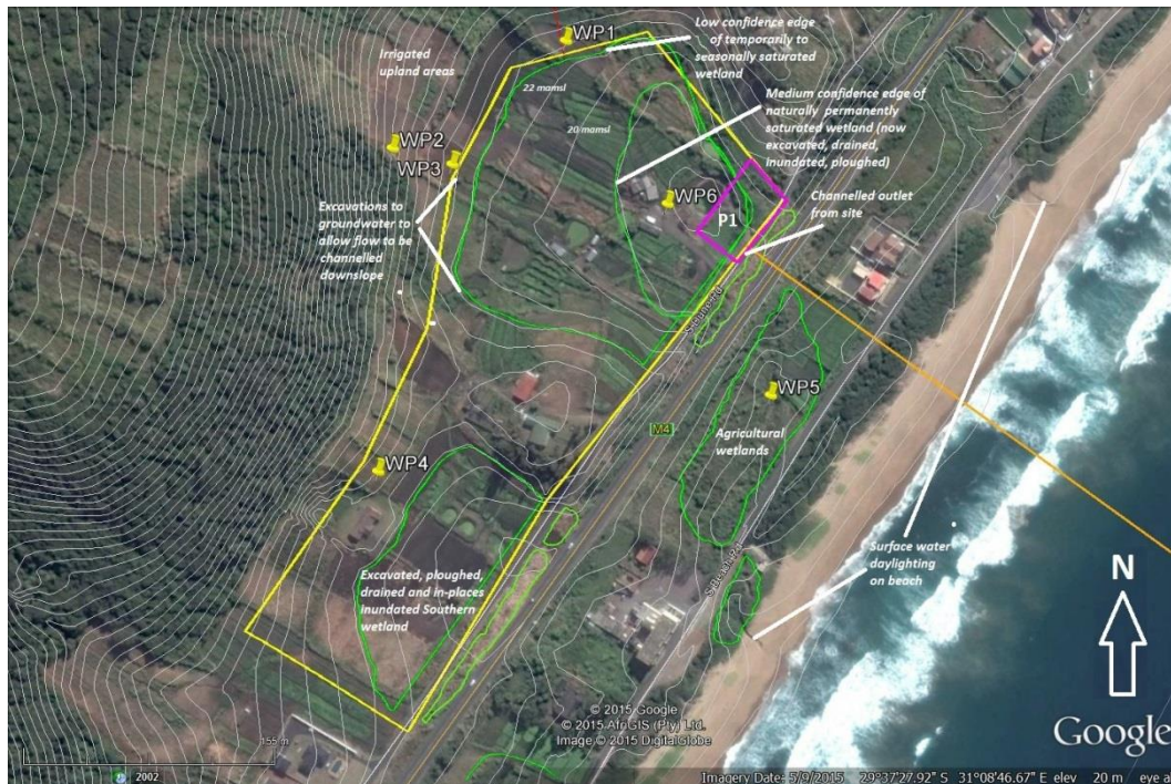
Figure 8-4: 2015 GOOGLE Earth image of the proposed desalination site, with 2 metre interval contour data and estimated extent of wetlands (green polygons) within the two basins in the desalination plant area. Purple polygon indicates proposed pump station site; the yellow polygon indicates the proposed desalination plant site boundary. “WP” prefix indicates augered points referred to in text.
