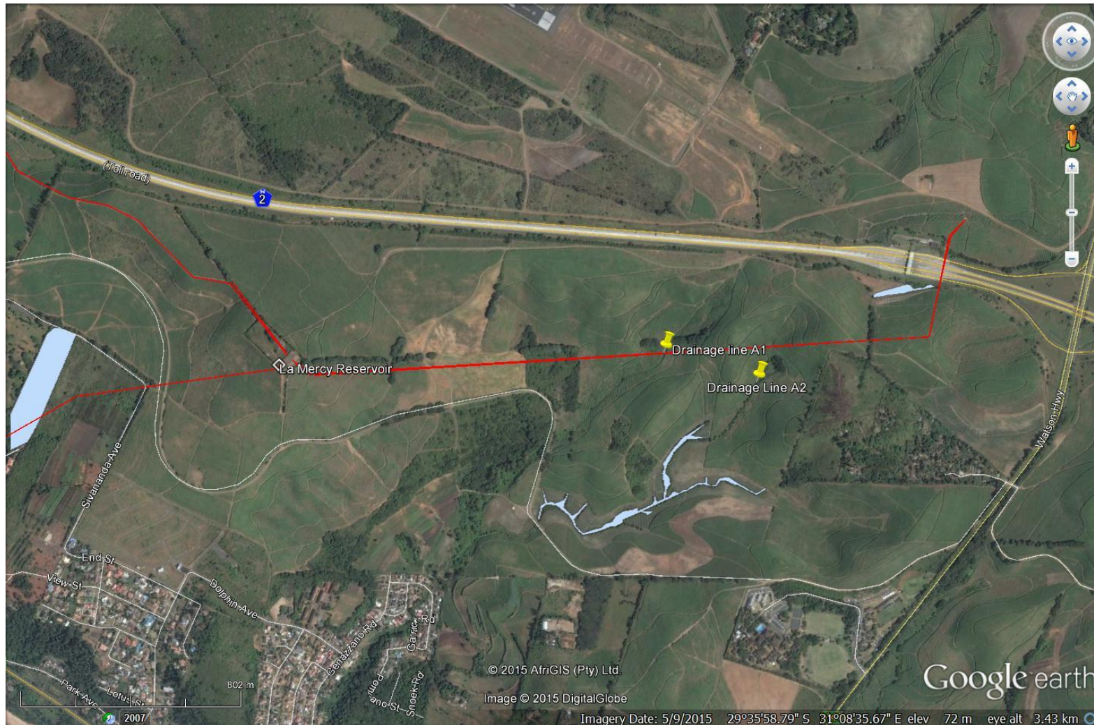
Figure 8-9: GOOGLE images of the proposed La Mercy to Waterloo pipeline route (red line) – La Mercy Reservoir - Bifurcation line. Note rotated North arrow. Blue polygons indicate mapped SANBI fine scale map data for Mdloti River wetlands and tributary.
