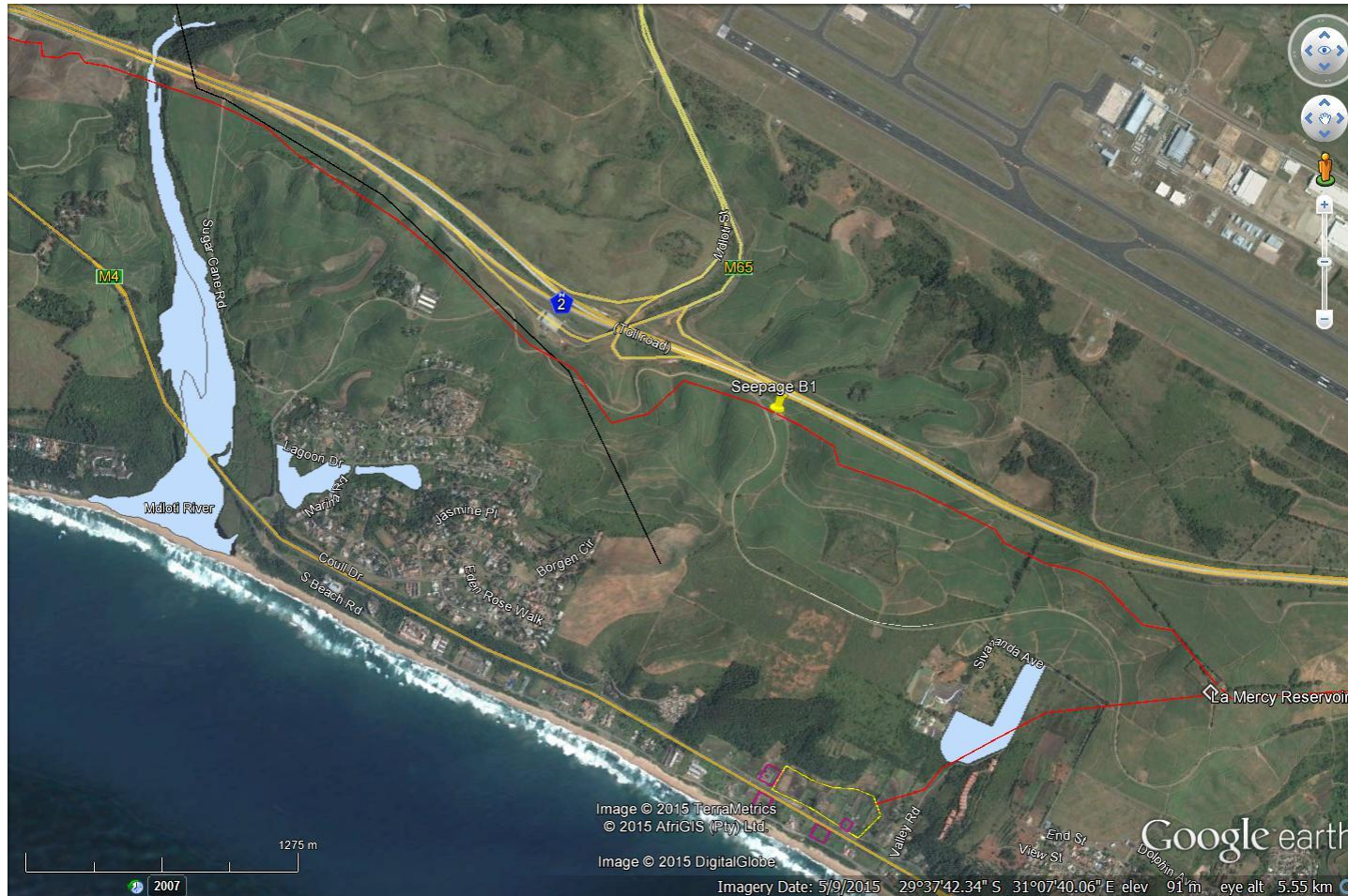
Figure 8-7: GOOGLE images of the proposed pipeline route (red line) –La Mercy Reservoir to Waterloo Reservoir route. La Mercy Reservoir to Mdloti River section. Note rotated North arrow. Blue polygons indicates mapped FEPA wetlands, also shown in SANBI fine scale maps
