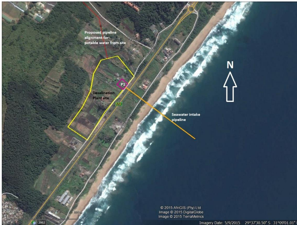
Figure 8-2: GOOGLE 2015 view of the proposed desalination facility at Tongaat, showing locations of proposed pump station (P1), desalination plant boundary (yellow polygon) and position of proposed seawater intake pipeline (tunnel) (orange).
