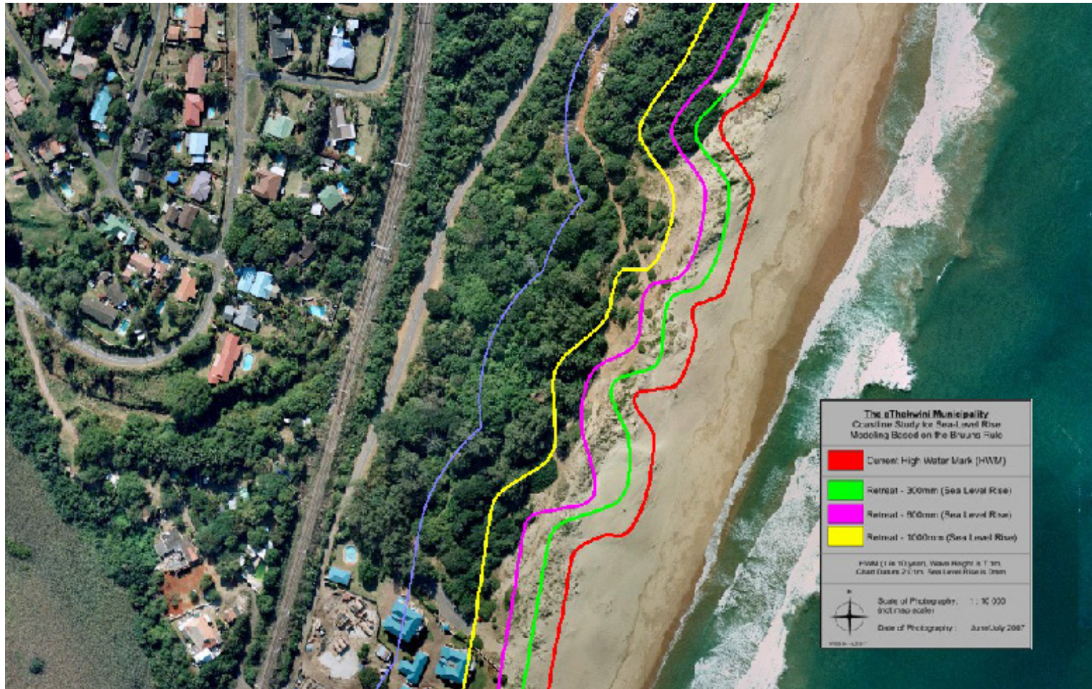
Figure 9.12 Image indicating expected marine inundation under accelerated SLR state as projected by eThekweni Municipality. Red: Current – High Water Mark (HWU); Green: Retreat – 300 mm (SLR); Pink: Retreat – 900 mm (SLR); Yellow: Retreat – 1000 mm (SLR) (eThkweni CVI and SLR GIS tool ; eThekweni Municipality)
