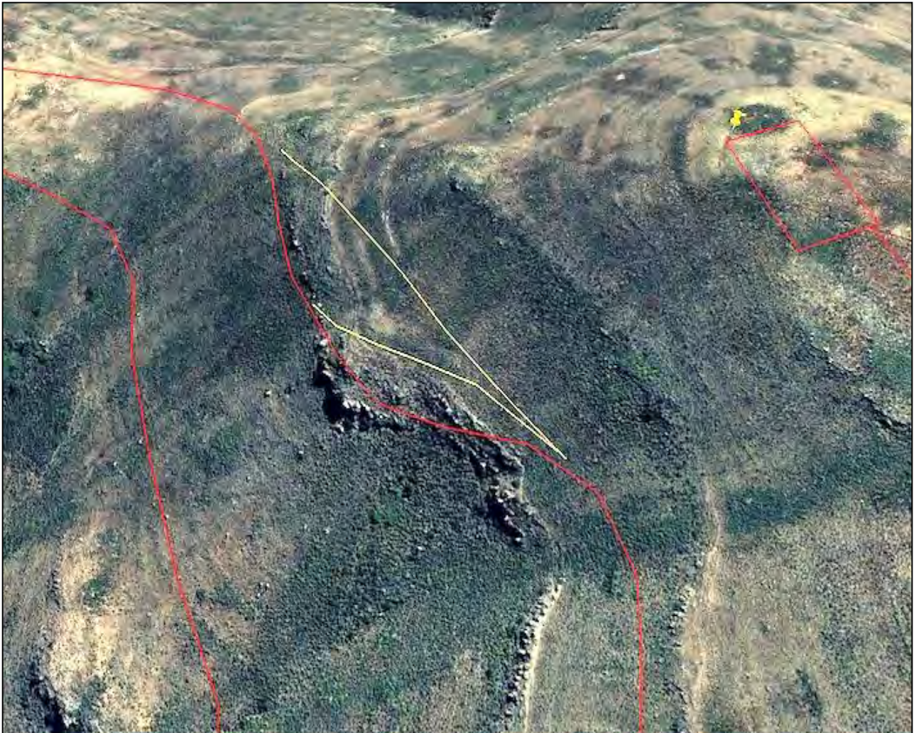
Figure 35: Proposed shift in position of internal access road between Turbines 28 and 29. (Road & crane pad boundary = red line, proposed re-alignment = yellow lines)
