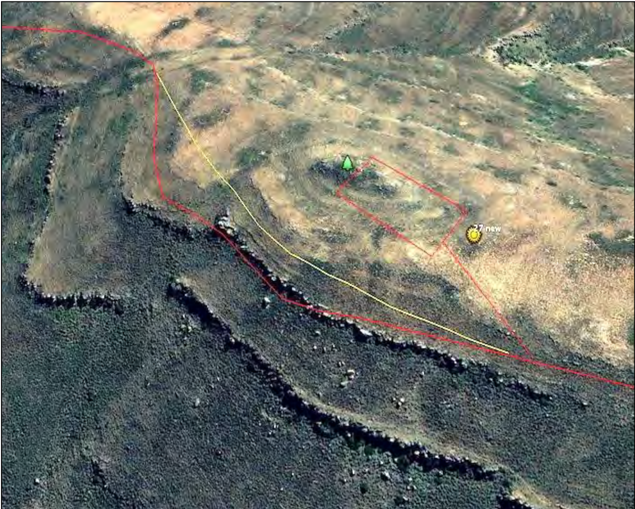
Figure 34: Proposed shift in position of internal access road between Turbines 28 and 29. (Road & crane pad boundary = red line, proposed re-alignment = yellow lines)
