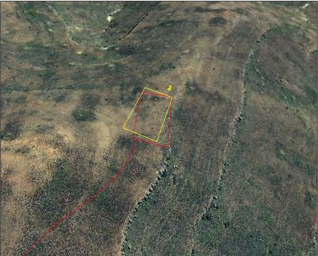
Figure 37: Proposed shift in position of crane pad at Turbines 35. (Road & crane pad boundary = red line, proposed re-alignment = yellow lines)
