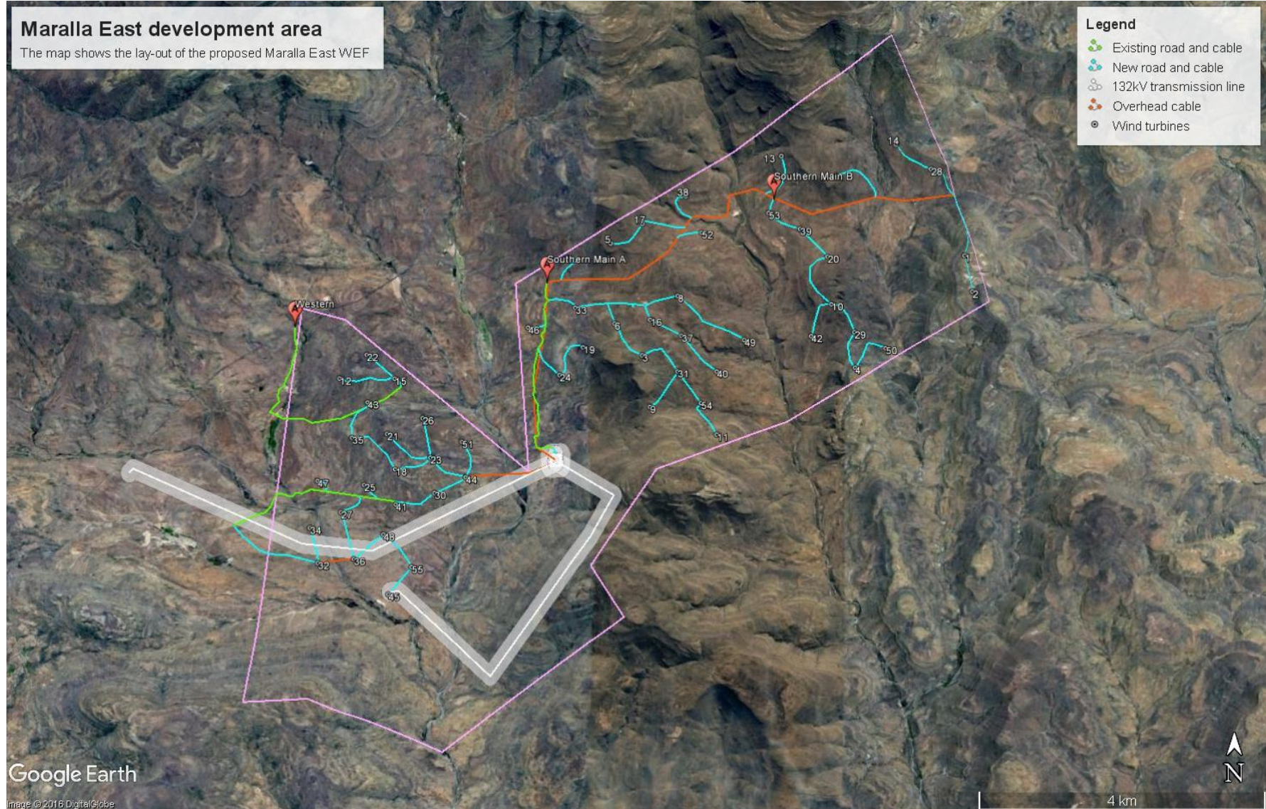
Figure 2: Lay-out proposed for the Maralla East WEF.
