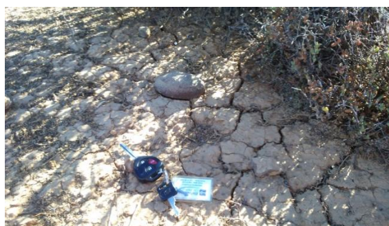
Plate 6 : Surface shrink-swell cracks on Depressional Pan
