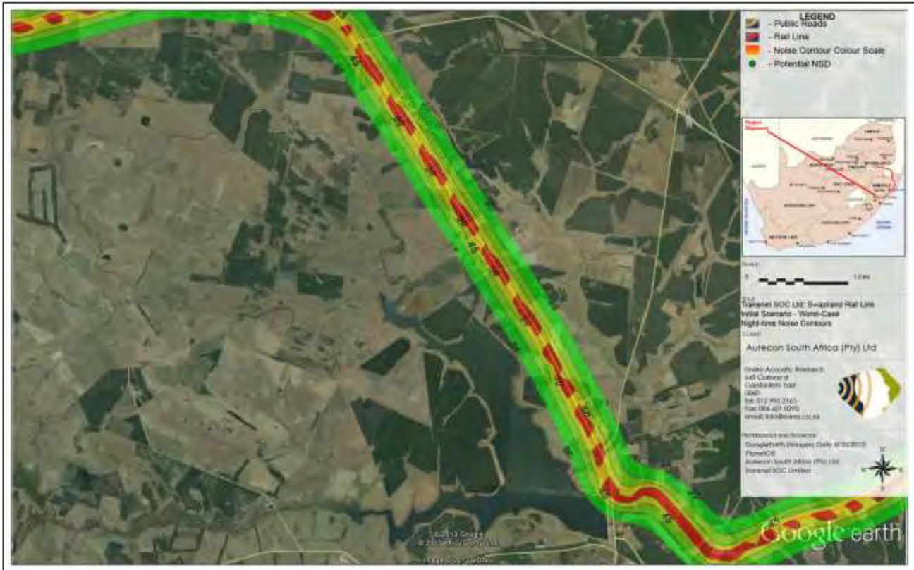
Figure 85: Projected initial scenario – Conceptual modelled worst-case night-time noise levels (no tone correction)
