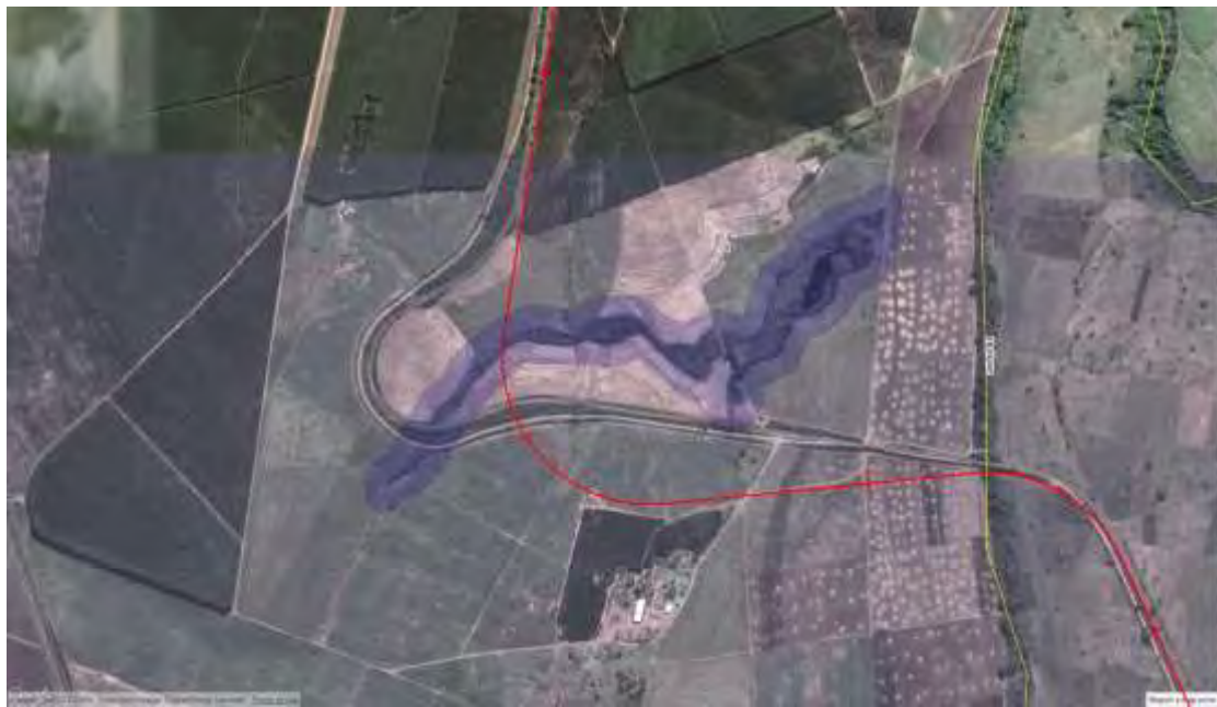
Figure 19: Freshwater marsh associated with the Hluhluwe River (S28.132219° E32.291549°) where the rail line alignment will be altered (red)
