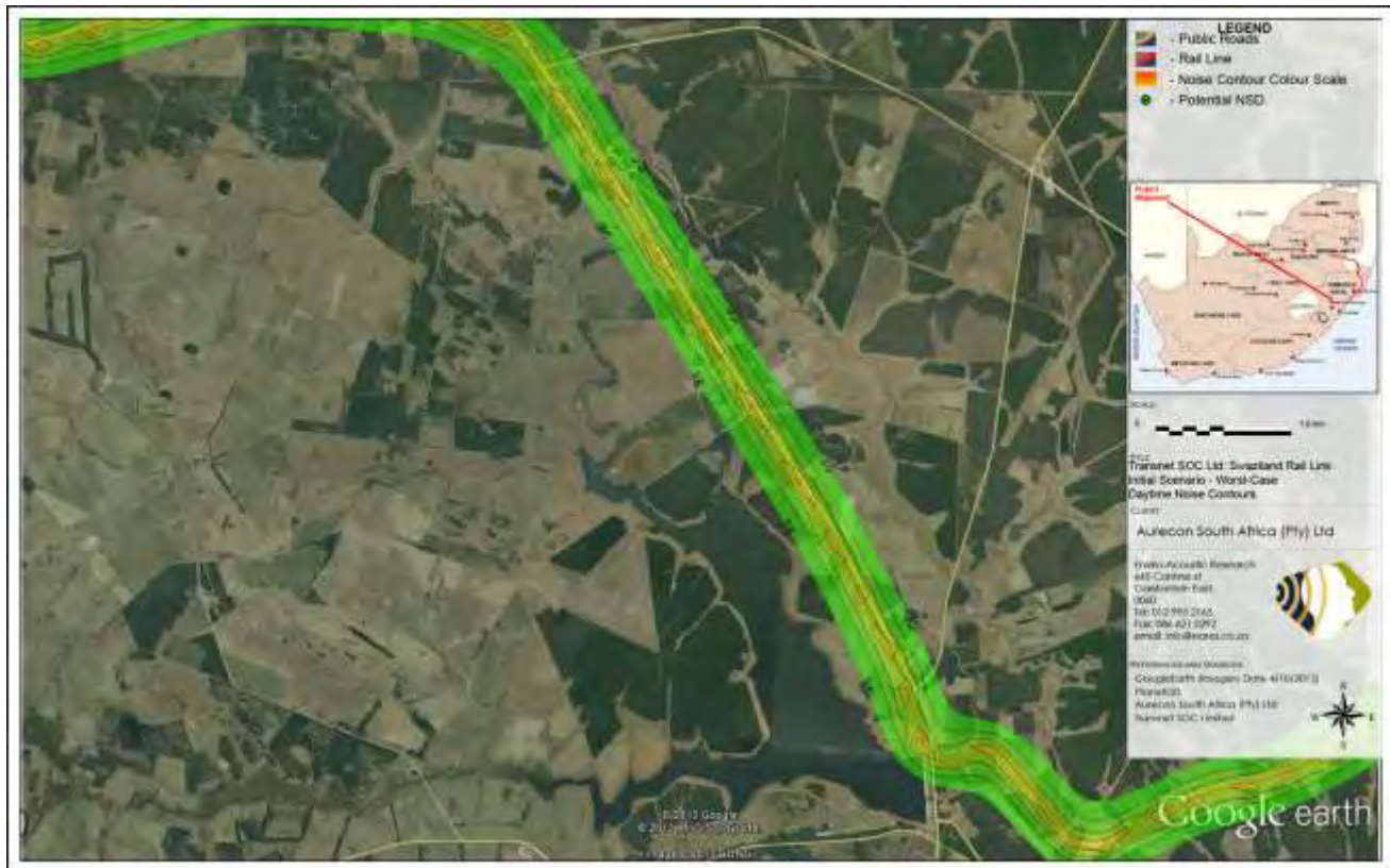
Figure 84: Projected initial scenario – Conceptual modelled worst-case daytime noise levels (no tone correction)
