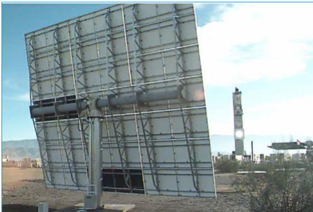
Figure 6-2 Rear view of Colon 70 heliostat
