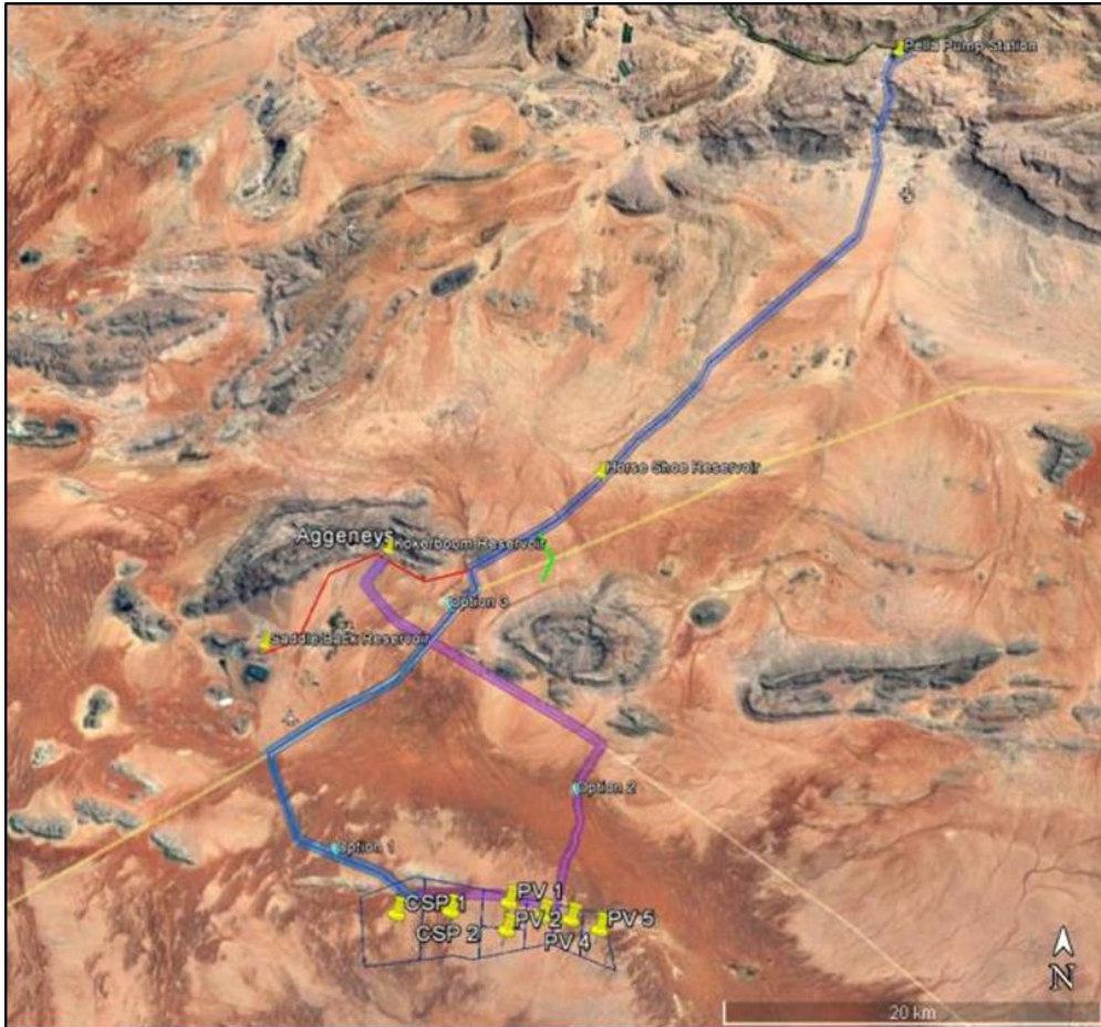
Figure 3: The water pipeline route from the Letsoai CSP to the Orange River. The water pipeline runs alongside the existing water pipeline from the Pelladri pump station on the Orange River to the mine at Black Mountain. An alternative option would allow the water pipeline to connect with the Kokerboom Reservoir at Aggeneys.
