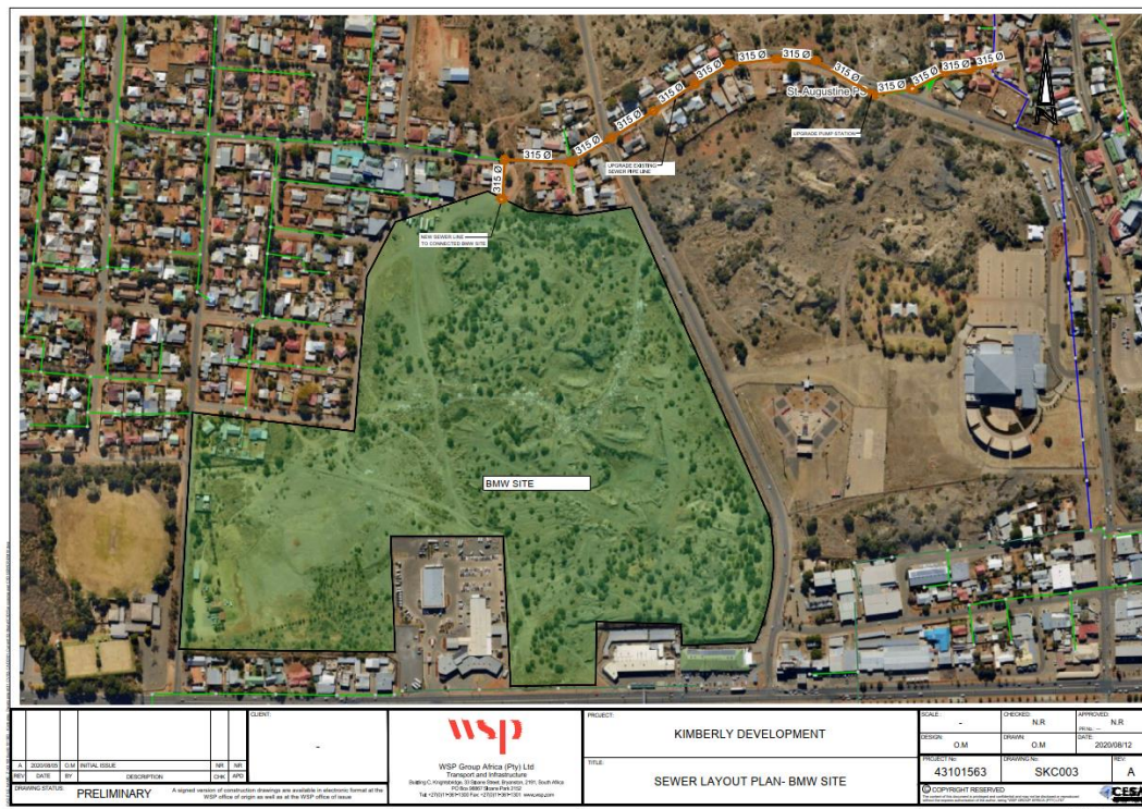
Figure 3: Proposed Sewerage Network at the BMW Site
