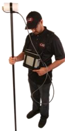
Figure 4: GSM-19T Proton Precession system in action.
