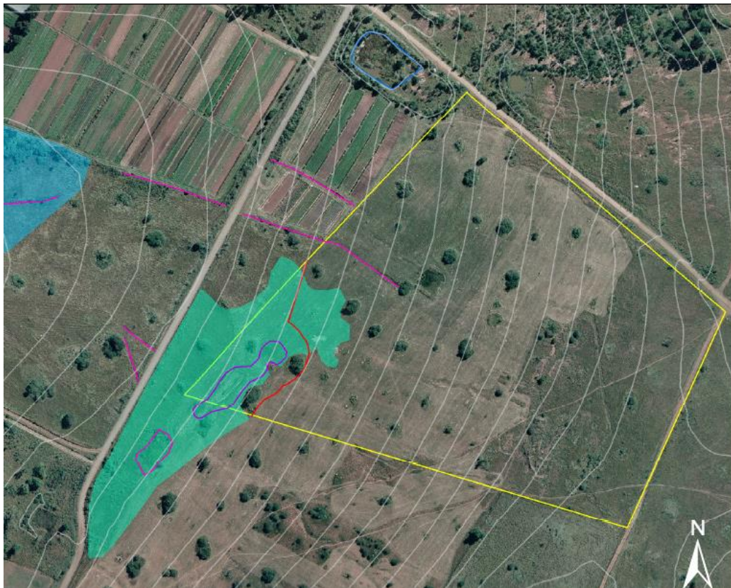
Figure 7: Image from wetland delineation study with artificial wetland in green and natural wetland in blue.
