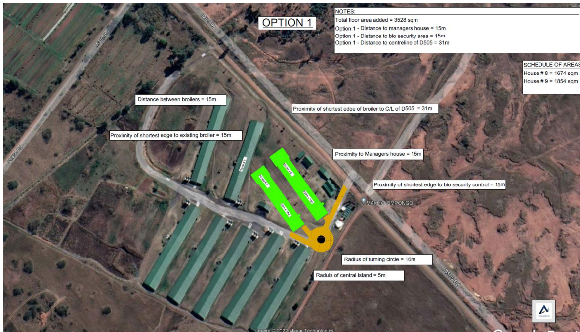
Figure 2: Figure showing layout of the proposed structures and the existing structures. (Layout can be found under Appendix A (2) (ii)).
