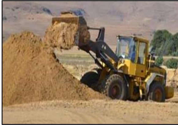
Figure 1-3: Typical Front-end loader stockpiling silica Gold Ore
