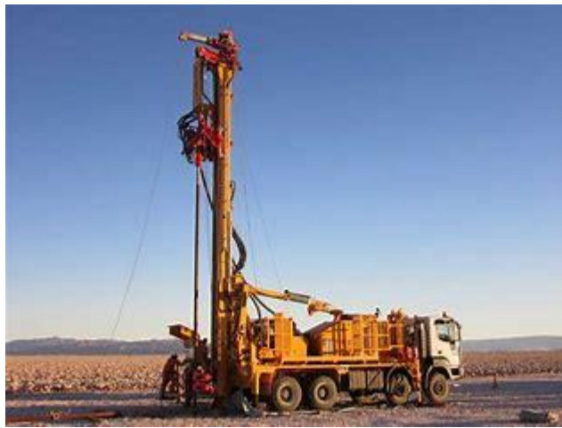
Figure 6: An example of a truck mounted RC drill rig.
