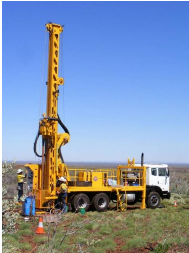
Figure 6: An example of a truck mounted RC drill rig.
