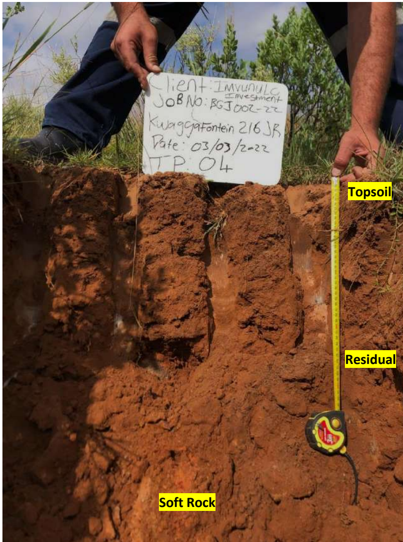
Figure 7: Typical test pit profile as observed on site.
