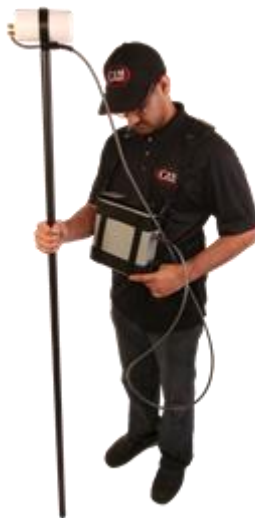
Figure 4: GSM-19T Proton Precession system in action.
