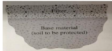
Figure 1: Definition of base material and filter material
