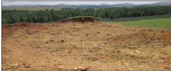
Figure 10-5: Dolerite gravel in borrow pit on sill
