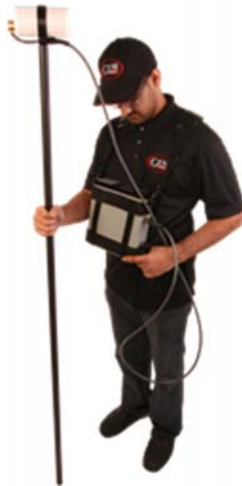
Figure 4: GSM-19T Proton Precession system in action.
