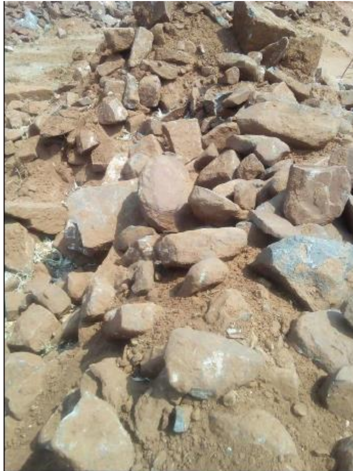
Figure 19: Loose boulders which is the limiting layer in the shallow southern area.
