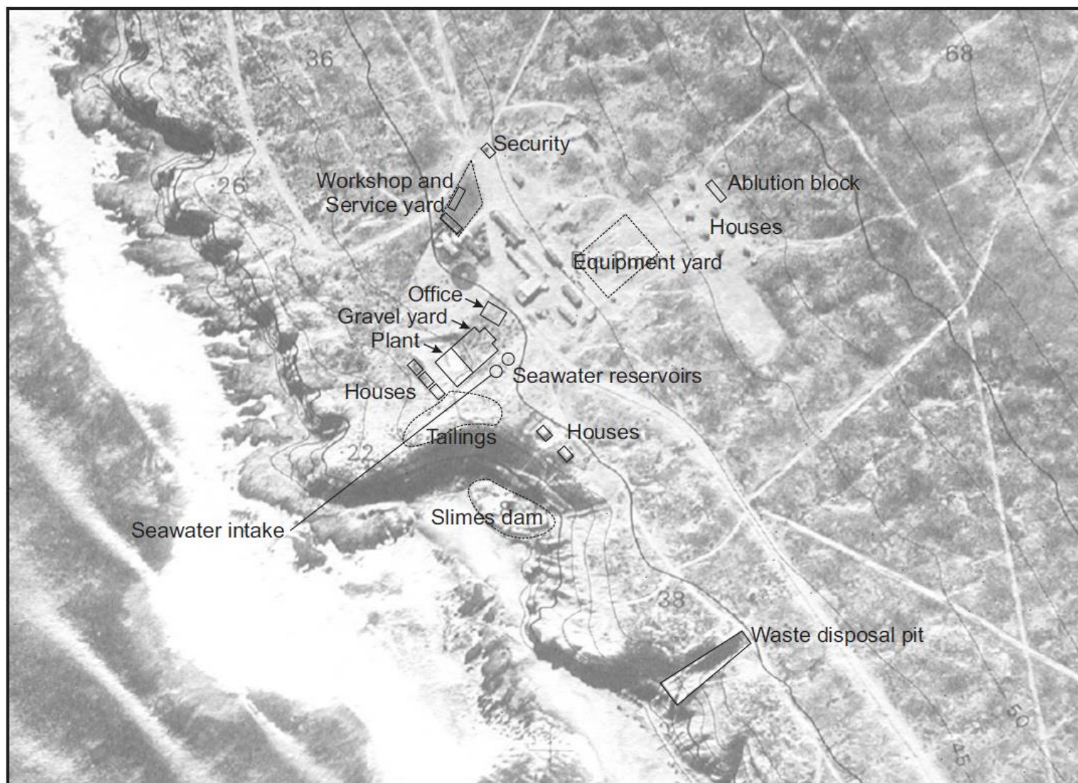
Figure 12: The facilities at De Punt, showing the location of the processing plant, gravel yard, tailings disposal and slimes dam. The waste disposal pit and housing, office and workshop facilities are also shown.
