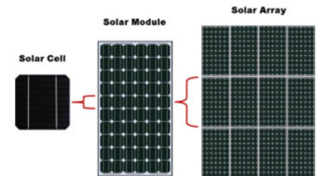
Figure 1: Overview of a PV cell, module and array/panel (Source: pveducation.com)
