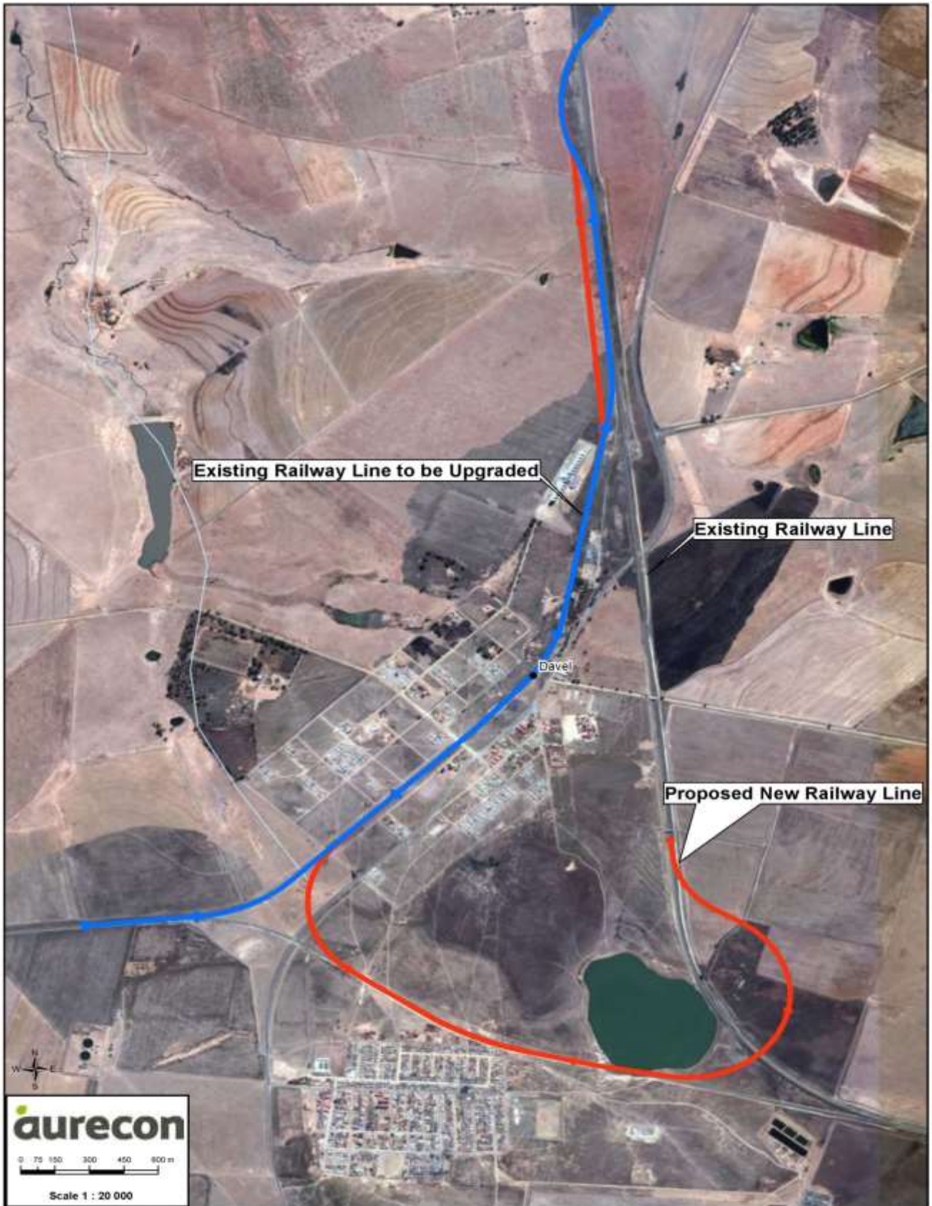
Figure 3: The Davel Rail Yard and associated connections. The red line indicates the new railway to be constructed. The blue line indicates the railway which is to be upgraded
