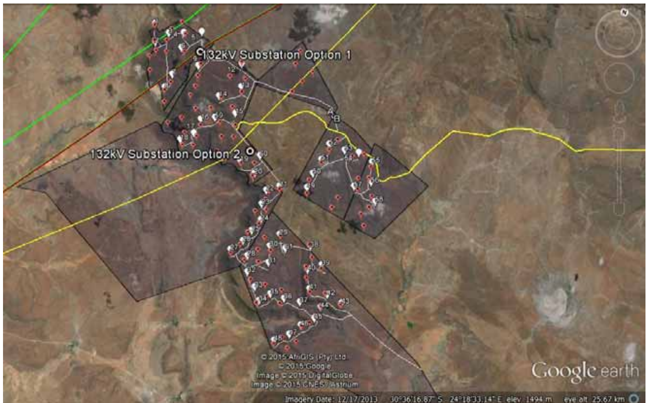
Figure 1: Proposed amended (preliminary) layout. Note: the red markers indicate the EA approved turbine positions and white markers indicate the new revised turbine positions. (Transmission lines are blue, red, green and yellow. Access roads are yellow and white).
