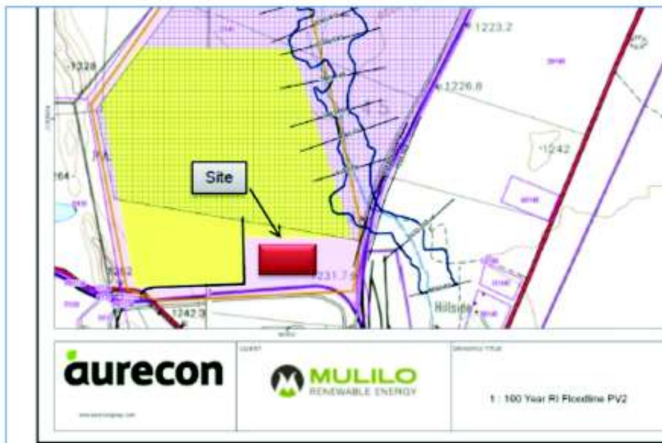
Figure 6. 1:100 year floodline along tributary of Brak River (Source: Aurecon 2012)
