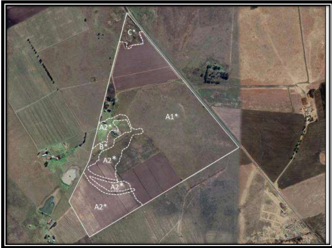
FIGURE 6: Preliminary geotechnical zones
