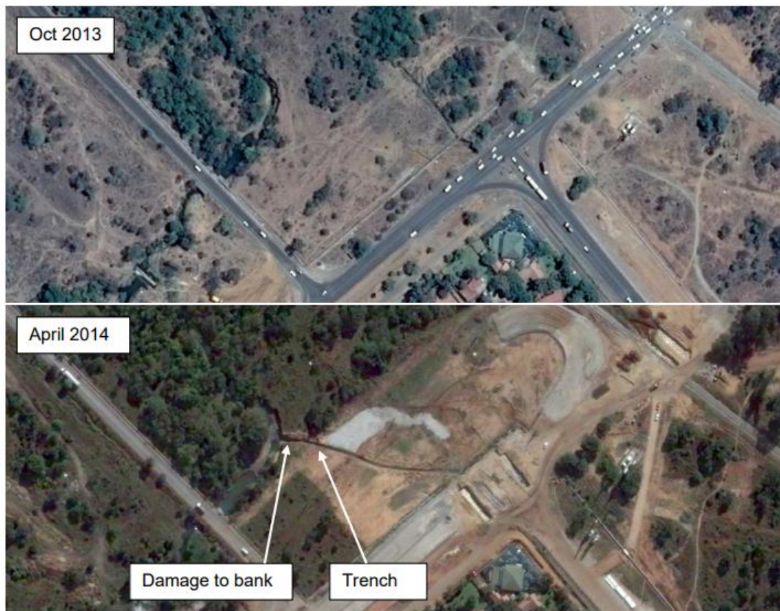
Figure 5-12 Two Google Earth images showing the changes that took place between Oct 2013 (top) and April 2014 (bottom), with specific emphasis on the stormwater diversion trench and damage to the eastern river bank
