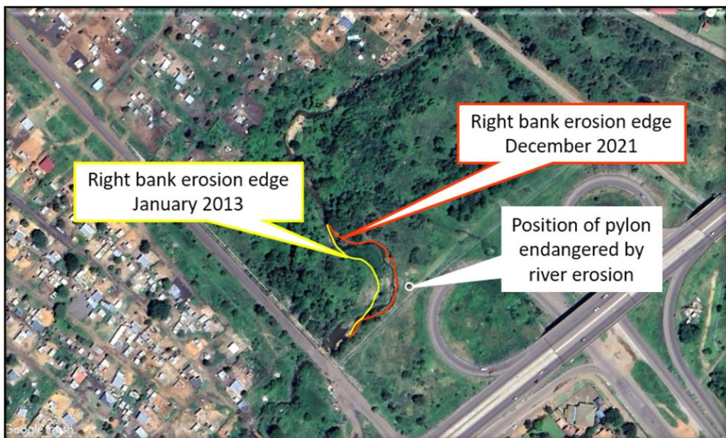
Figure 2-4 Riverbank erosion progression
