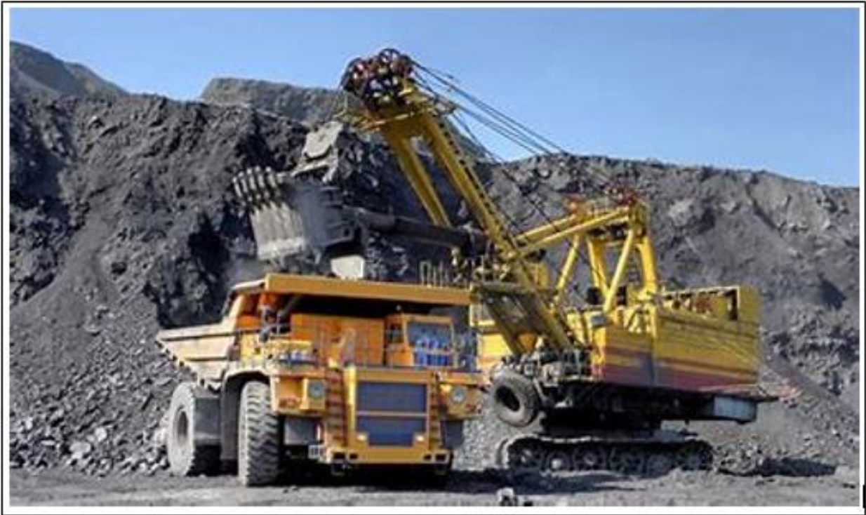
Figure 4: Demonstrating the truck and shovel method.
