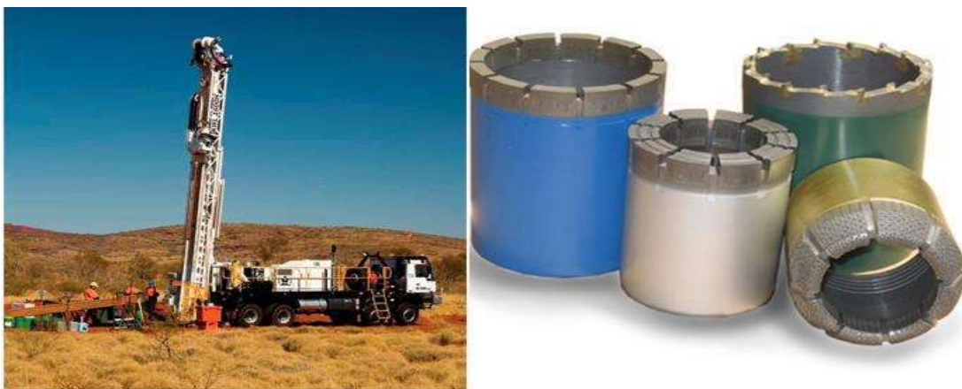
Figure 6: Typical example of Diamond Core drill rig and drill bits.
