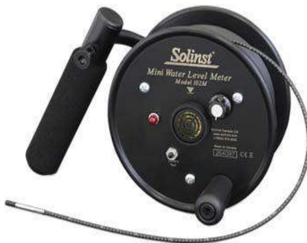
Figure 2: Solinst Dip Meter used to sample borehole water.
