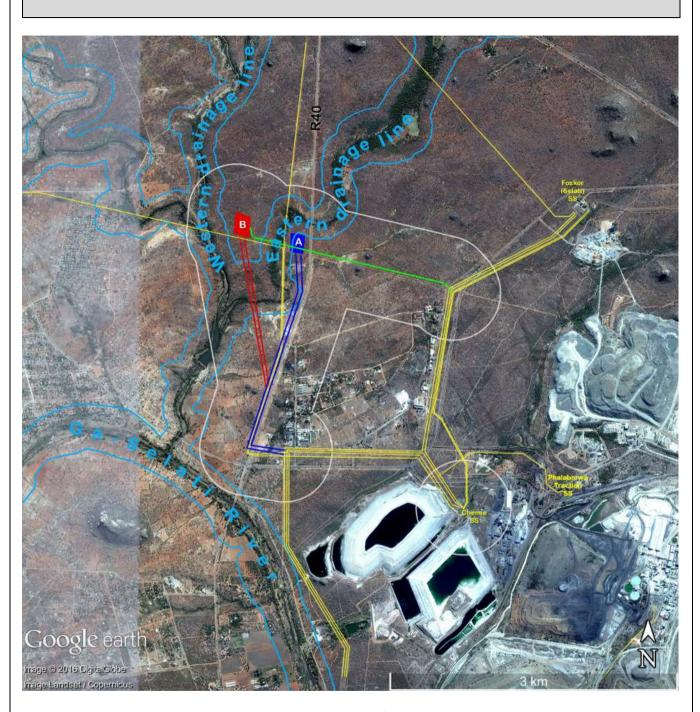
Dark blue: Alternative A (Preferred Alternative) Red: Alternative B Green: Connection to existing Chemie-Selati power line Yellow: Existing power lines White lines: 1km zone around the proposed developments, including the decommissioning of the old Chemie substation in the south-east; Light blue: 100m buffer zone around prominent drainage systems.
