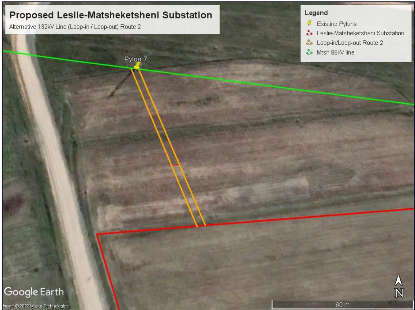
Figure 10: Alignment of the proposed/preferred powerline route
