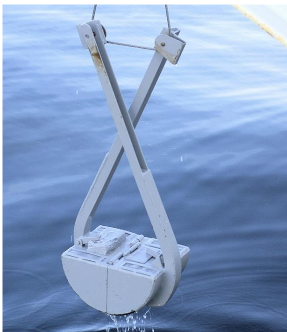
Figure 6.8. (Left) A Van Veen grab works like a claw to grab sediment containing macrofauna from the seafloor. (Right) Example of a corer. Source: British Ocean Sediment Core Research Facility.
