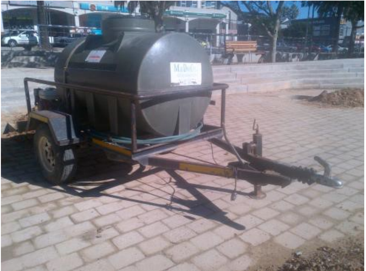
Figure 14: Indicating a mobile water cart
