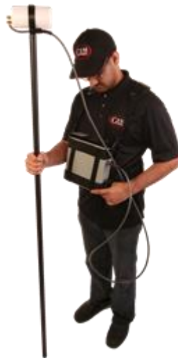
Figure 3: GSM-19T Proton Precession system in action.
