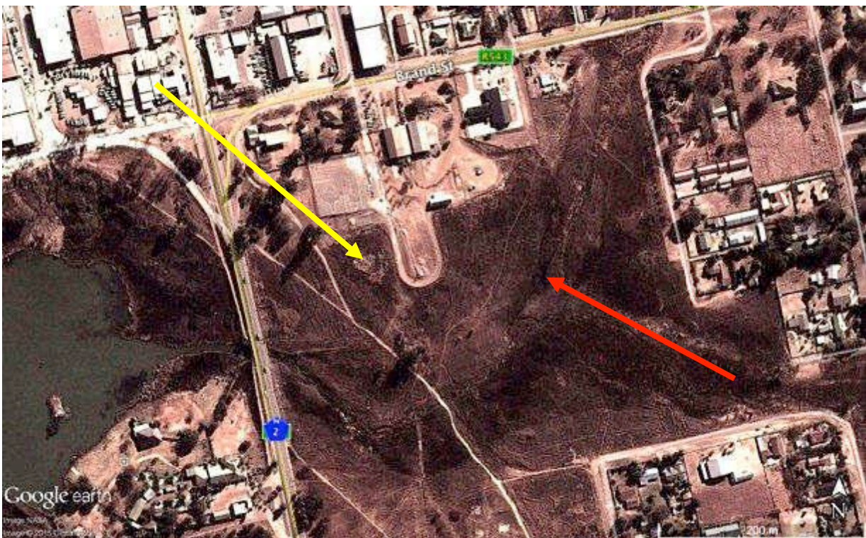
Figure 14 Google Earth image (2011/07/20) with the potential seepage areas (yellow arrow) very evident as artificial modifiers and without signs of a potential seepage wetland in the east (red arrow)
