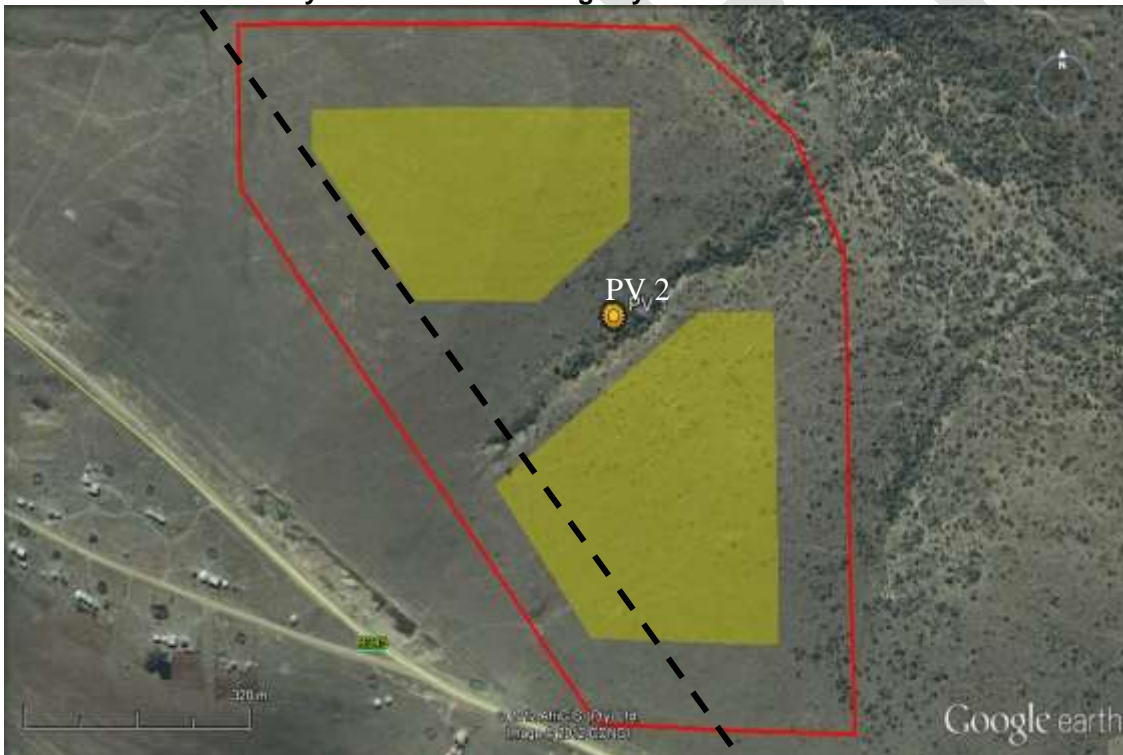
Figure 1-19: An aerial photo shows the trees rich drainage system. The yellow polygons represent the solar panel's footprint. The dashed line represents the existing power line layout.
